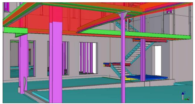
For this to work and save time, the rebar cages had to be fabricated for the full six stories off site then delivered and swung into place between the steel frames. This meant that the steel frame and rebar had to be completely coordinated. GPLA was able to fully detail both systems in their model and the rebar cages were able to be swung into place after the steel was erected.
